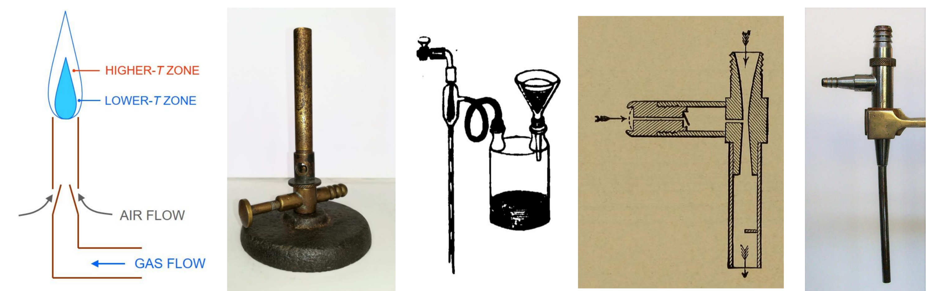
Illustration of two applications of the Venturi effect: the Bunsen burner (left) and the Venturi vacuum pump (right) [6, 10-11].
