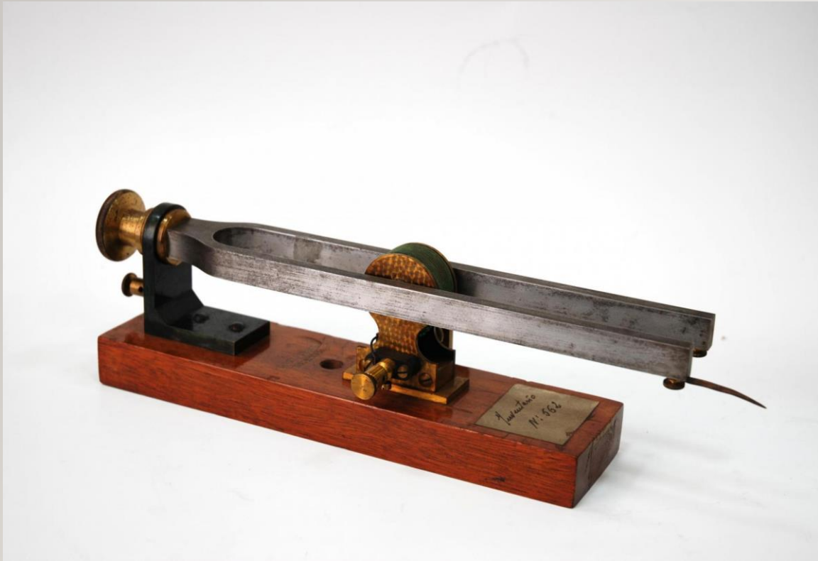
Chronograph tuning forks with electromagnetic drive
