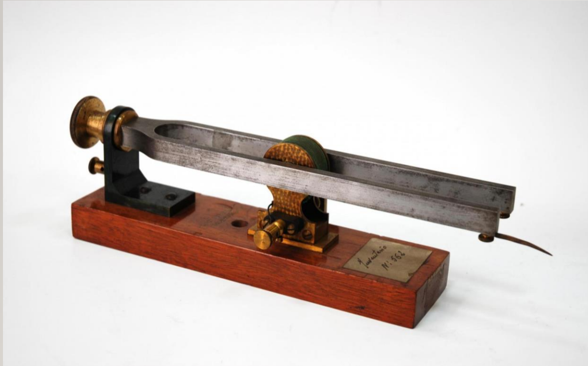
Chronograph tuning forks with electromagnetic drive, by Max Kohl, Germany, acquired in the 1906.
