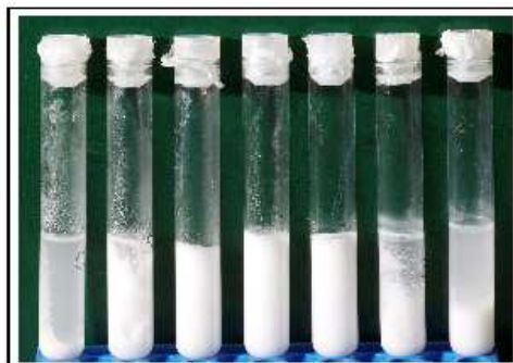
Fig. 3.7: Lysozyme solutions ( 20 \text{ mg/ml} ) in PBS buffer with increasing TFE content (0, 5, 10, 15, 20, 30, 50 % from left) after incubation at 65^\circ\text{C} for 20 days.
