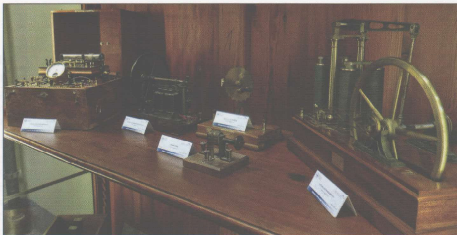
Fig. 4 Electromagnetic instruments in Case 4: electrotherapy apparatus; two magneto-electric motors; interrupter and in foreground a commutator. Photo: Jean François Loude.
