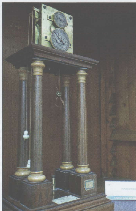
Fig. 5 Large Hippi Chronoscope without its glass cover, introduced in 1848 by the clockmaker Matthäus Hippi for use in experimental psychology. Photo: Jean-François Loude.
