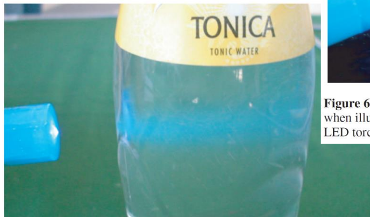
Figure 5. Blue light emitted by the quinine in commercial tonic water when illuminated with UV light produced by a portable LED torch.
