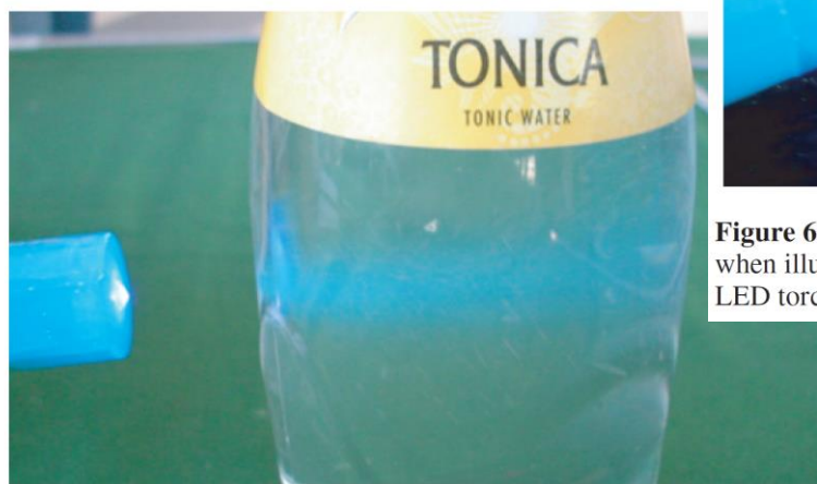
Figure 5. Blue light emitted by the quinine in commercial tonic water when illuminated with UV light produced by a portable LED torch.
